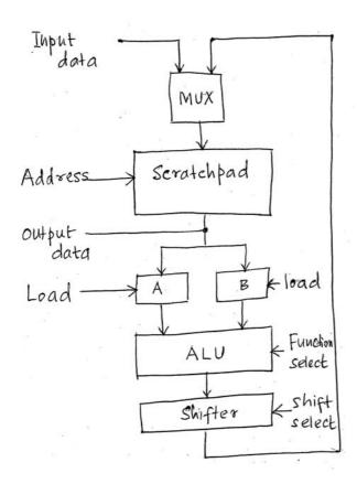
The processor consists of 64 registers of eight bits each.
